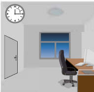
Light switches off automatically after the stand-by period elapses.
