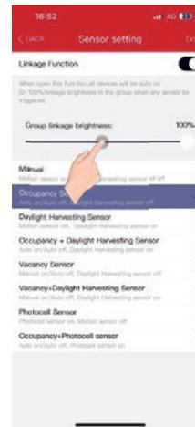
3. Set the group linkage brightness in the sensor settings interface. Must click "Done" to save the linkage function
