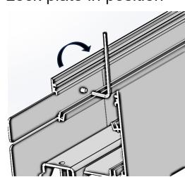
Insert Joint lock holder to brackets
