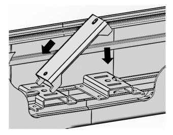
Fix lock holder to brackets by 2 screws
