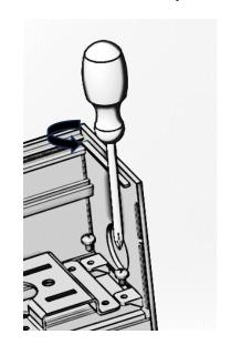
Insert Joint plate to housing
